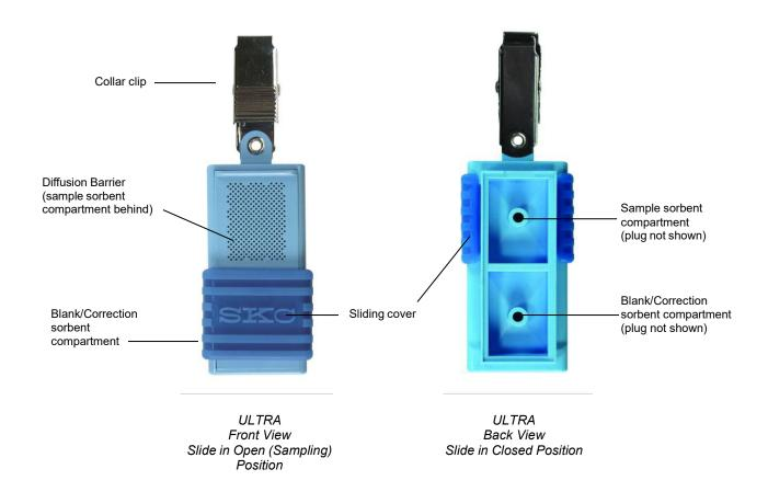
Figure 1. ULTRA Passive Sampler with Blank/Correction Compartment
